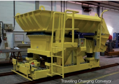
Travelling Charging Conveyor
